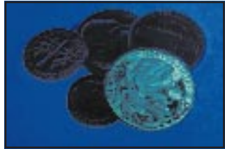
This is a coin treated with invisible coin lacquer, viewed under ultraviolet light.
