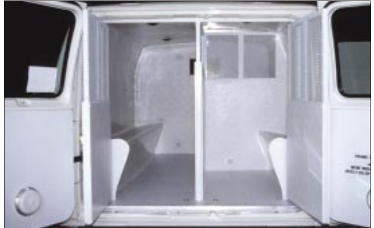
Optional dual inner security door allow for better control when unloading prisoners from the PTV100. (Option No. PTV-6)
