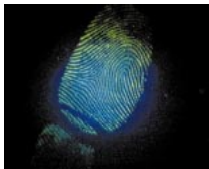
Cyanoacrylate print dye-stained with ardox and viewed with the Melles Griot Omniprint 1000A
