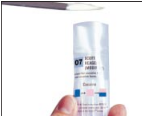
Step 1. After removing the clip, insert a small amount of suspect drug into the test pouch.
