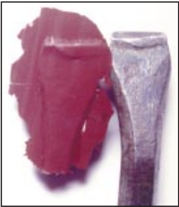
Mikrosil™ used to cast a door jam where a pry bar was used to gain entry.
