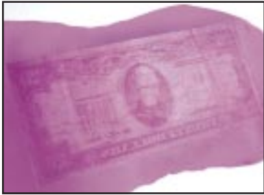
This is an actual cast of the ink depth of a 20 dollar bill.
