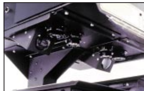
This is a close-up of the unit's turret-mounted lenses and its dual-quartz light source.
