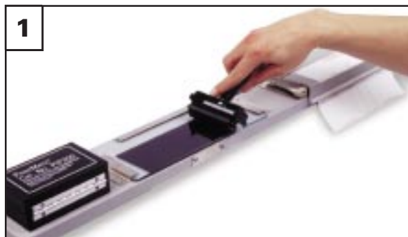
1 The operator applies ink to the slab with the No. PIP100.
