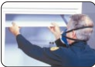
The main cabinet prefilter can be changed easily between cases to prevent cross-contamination.
