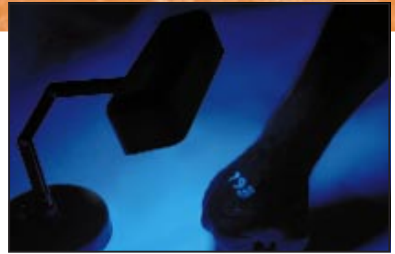
Invisible skin marking ink is invisible in natural light and highly fluorescent when exposed to ultraviolet light.
