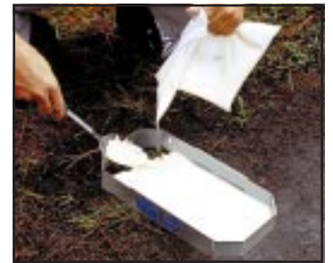
Step 4: Pour into impression.* *Optional accessories pictured.
