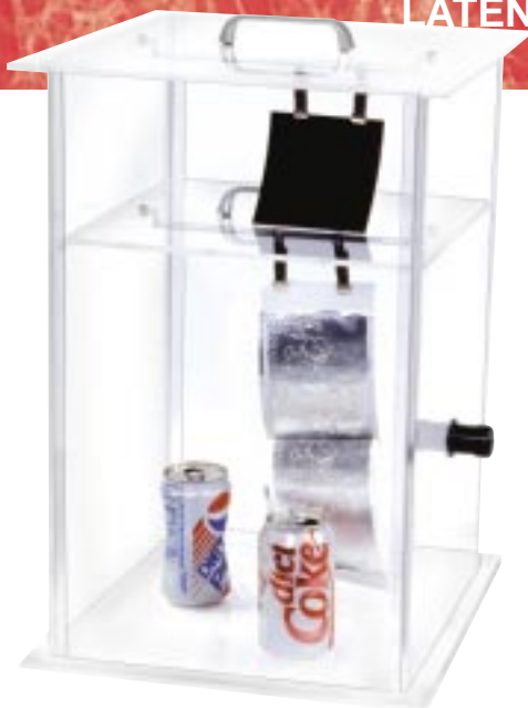
The portable cyanoacrylate fuming chamber, No. CNA900, is assembled and in use.
